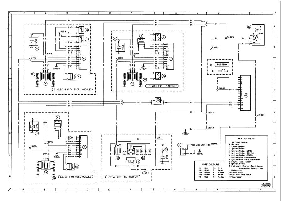
Diagram 1a: Ignition system - carburettor models
